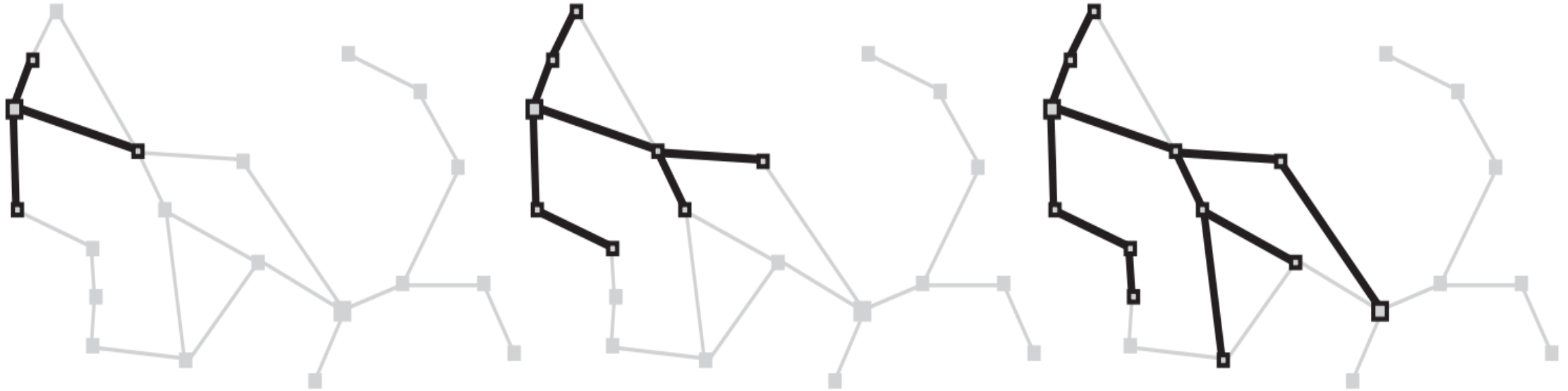
Figure 3.8 A sequence of search trees generated by a graph search on the Romania problem of Figure 3.2. At each stage, we have extended each path by one step. Notice that at the third stage, the northernmost city (Oradea) has become a dead end: both of its successors are already explored via other paths.
